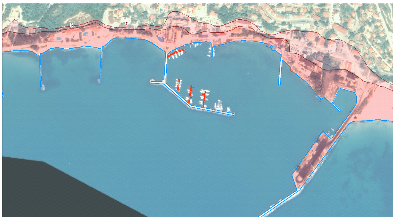
Fig.7. The possible inundated areas (3 m and 7 m) and vulnerable objects.
