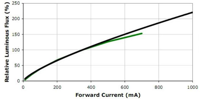
Fig.6. Typical LED flux-current characteristics [12], used to control the individual LED flux intensities in Eq.1.1
