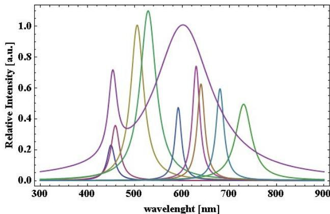
Fig.2. Relative Intensity spectra of different discrete LED sources
