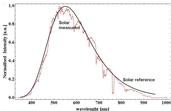
Fig.1. Measured Sun spectrum at ground level (dotted line) and the theoretically equivalent  $T=5500K$  black body emission spectrum (solid line)(both normalized to their maxima)
