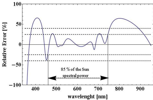
Fig.4. Relative Error of the LED synthesized light source spectrum compared to the Sun reference spectrum
