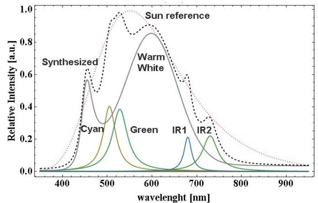
Fig.3. Relative Intensity spectra of the synthesized LED source (dashed line), the used in its construction commercial LEDs (solid lines) and the Sun reference spectrum (dotted line)
