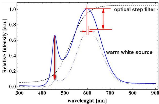
Fig.5. Effect of applying a step optical filter in front of the used discrete white LED source
