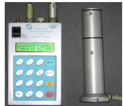
Fig.2. View of the Liulin-5 instrument. In the left part is seen the electronic block, while in the right is the detector module. The first detector of the telescope is at the bottom of the figure, the second is in the middle where the black line is seen, the third is at the top
