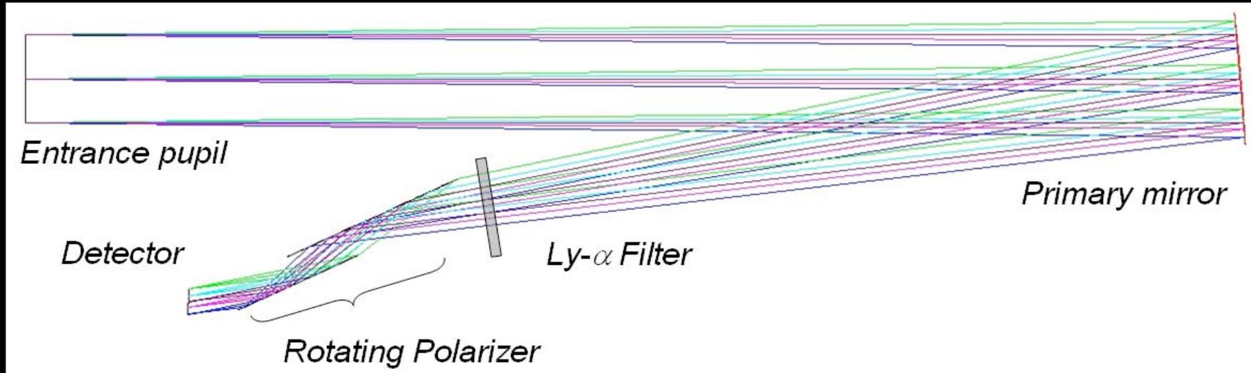
**The Lyman Alpha and O VI Coronal Imager schematic set-up. Note that the filters are in a five positions filter wheel to access H I 121.6, 102.5 and 97.2 nm and O VI 103.2 and 103.7 nm.**
