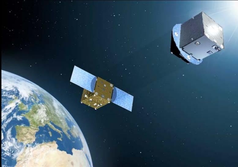
A coronagraph with the external occulter on one spacecraft and the optical instrument on the other spacecraft, ~150 meters from the first one
