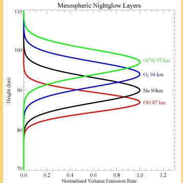
4. Neutral atomic oxygen (O(<sup>1</sup>S)). Line at 557.7 nm. Most comes from the mesosphere near 96 km via the three-body Barth reaction
