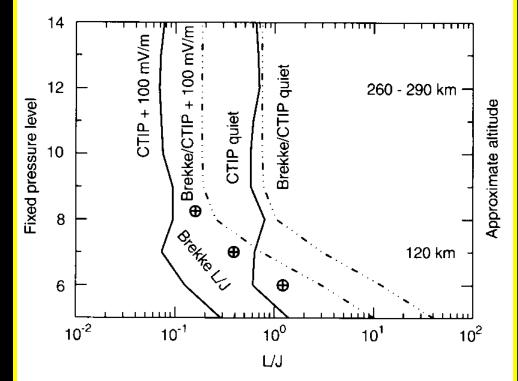
Fig. 3. Plot of the ratio of Lorentz forcing to Joule heating against height at latitude  $70^{\circ}$ N, longitude  $162^{\circ}$ E, Day 1. The *two solid lines* show the coupled model results for (a) quiet atmosphere, and (b) during the 100 mV/m enhanced electric field. The *broken lines* show results from the extrapolation of the Brekke formula, Eq. (4), for both quiet and enhanced atmospheres, whilst the *three discrete points* are the Brekke results
