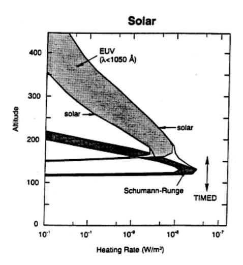
Altitudinal profiles of heating rates due to solar EUV and UV absorption. The shaded regions indicate the range of variations with solar activity. The TIMED Mission investigates the region of maximum energy deposition.
