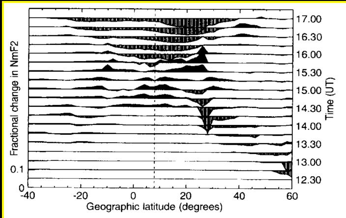
Fig. 5. Change in NmF2 (the density of the F2 peak), relative to steady-state conditions. The format of the plots is identical to that of Fig. 1
