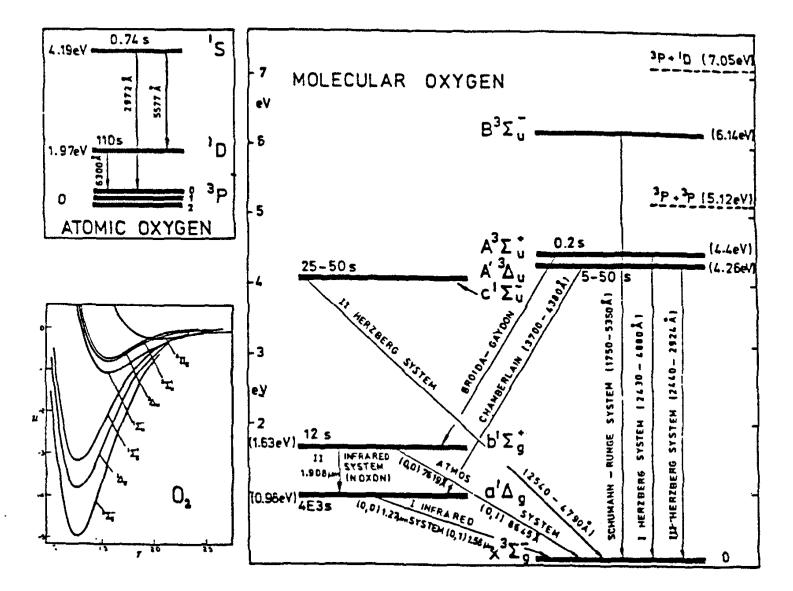
Fig. 6. Energy level diagram of molecular and atomic transitions of oxygen [from Greer et al. 1987]
