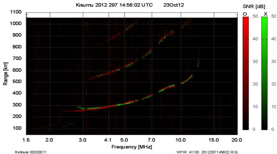
Figure 4: One of the first ionograms recorded with Maseno VIPIR ionosonde. The plot shows signal strengths in dB for ordinary (red) and extraordinary (green) waves
