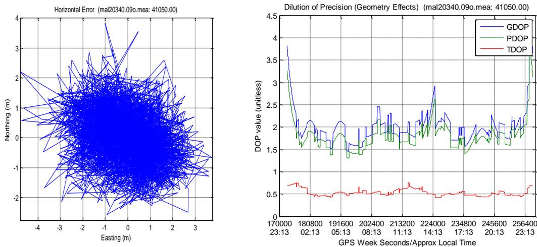
Fig 4 (a)Horizontal error: 2m Northing; 3m Easting (b) Dilution of Precession
