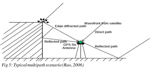
Signal interference at the antenna due to multipath causes fluctuations that can resemble scintillation, but these fluctuations are not caused by the ionosphere
