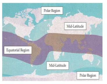
Fig 1: Equatorial region scintillation belt (www.vs.afrl.af.mil)
