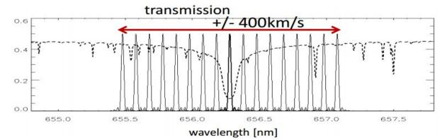
By using a liquidcrystal Lyot filter
