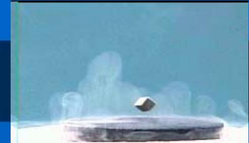
A superconductive disk on the bottom, cooled by liquid nitrogen, causes the magnet above to levitate. The floating magnet induces a current, and therefore a magnetic field, in the superconductor, and the two magnetic fields repel to levitate the magnet.
