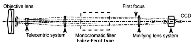
Fig. 3. Schematic of the optical system of a telescope in the FMT 2 . Every five telescopes have almost the same structure.
