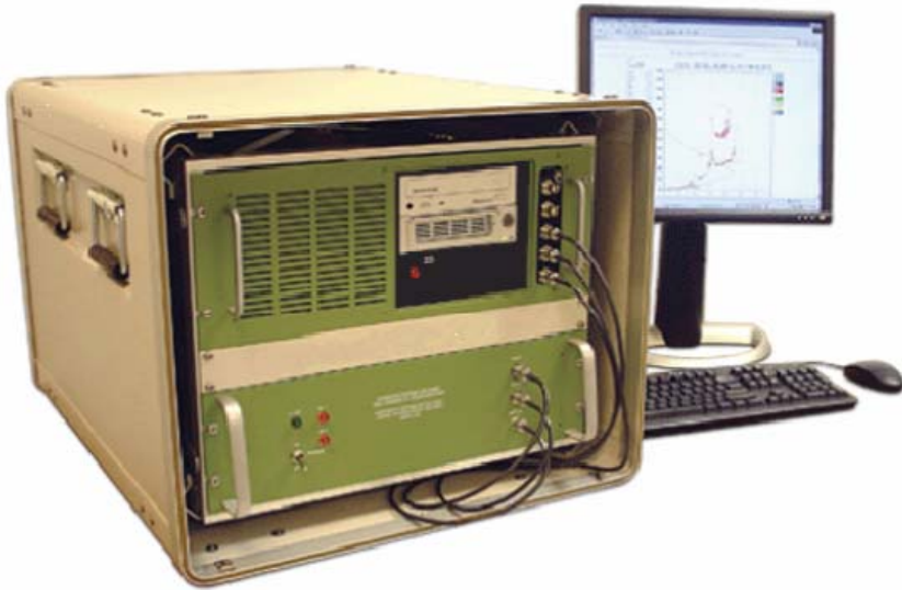
Fig.6: Portable Digisonde Sounder
