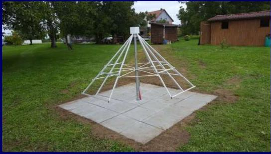
New Callisto spectro-polarimeter in Landschlacht, Switzerland. Replaces instrument from Bleien observatory, a facility of ETH Zurich which will be closed due to retirement of the PI Chr. Monstein
