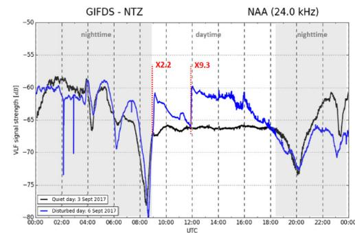
Figure 1: GIFDS measurements at the Neustrelitz station on September 3 and 6, 2017 showing severe Flare activity on 6 September 2017 (for further details see Berdermann et al., 2018).
