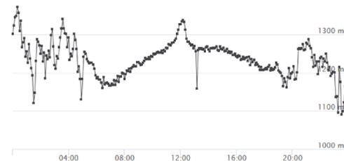
Figure 1: VLF amplitude variation during the solar eclipse on the 21 August 2017 (EST) recorded by the SOFIE receiver HV1 in Huntsville Alabama: HV1 measures the VLF signal transmitted by NML (LaMoure / North Dakota).
