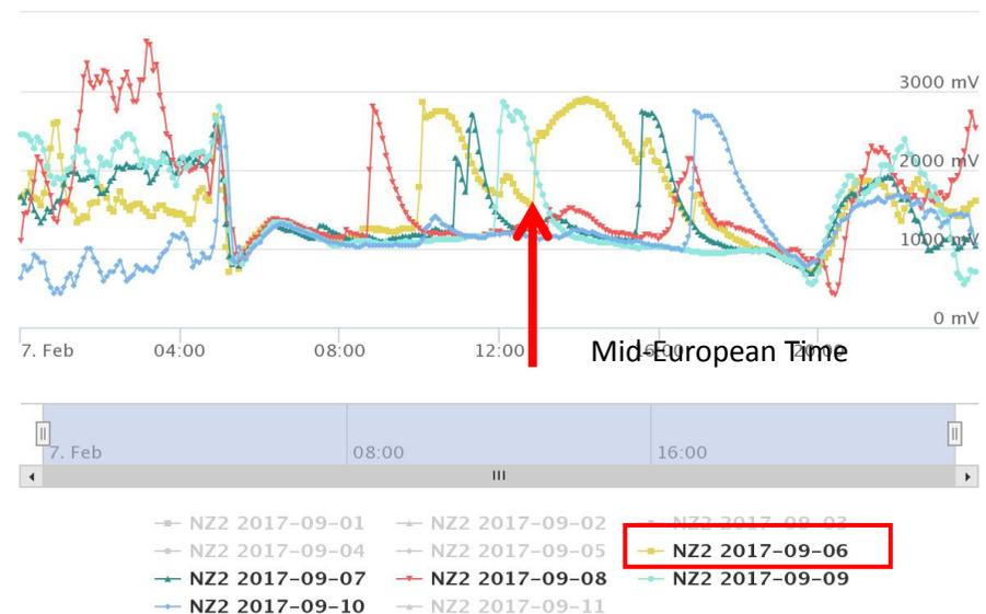
VLF signal strength measurements via SOFIE receivers in Neustrelitz revealed numerous solar flares from September 6 -10, 2017. The X 9.3 solar flare on 6 September 2017 causing an impact on GNSS positioning (see previous slide) is indicated by an arrow.
