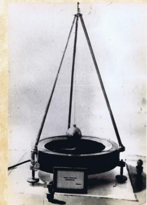
Fig. 2 Fr. Ricart's 1869 design of a pendulum seismometer, now known as a seismoscope.
