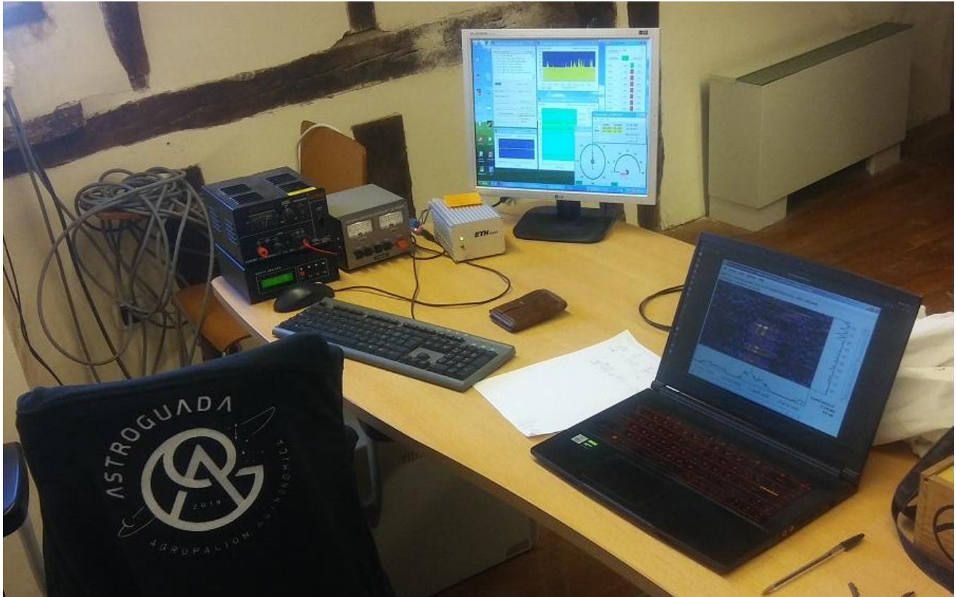
Fig. 11: From left to right: Antenna tracker and power supply, CALLISTO, monitor and notebook for data analysis in Sigüenza, Spain.
