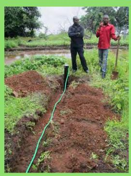
Layout the cable and put the sensor in a right position, vertical!!
