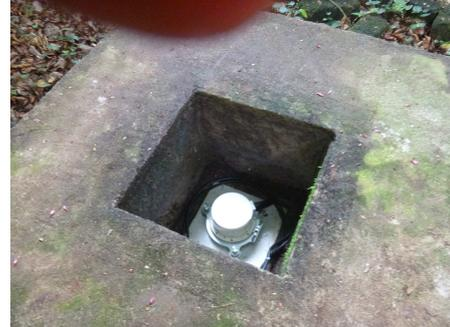
The round thing is the sensor. It is set in a heavy structure that was built by Yumoto/Kakinami/Maeda in year 2006 with the help of local laborers. It is set in a jungle environment, which keeps off a lot of sunlight. So diurnal temperature variation is not large.
