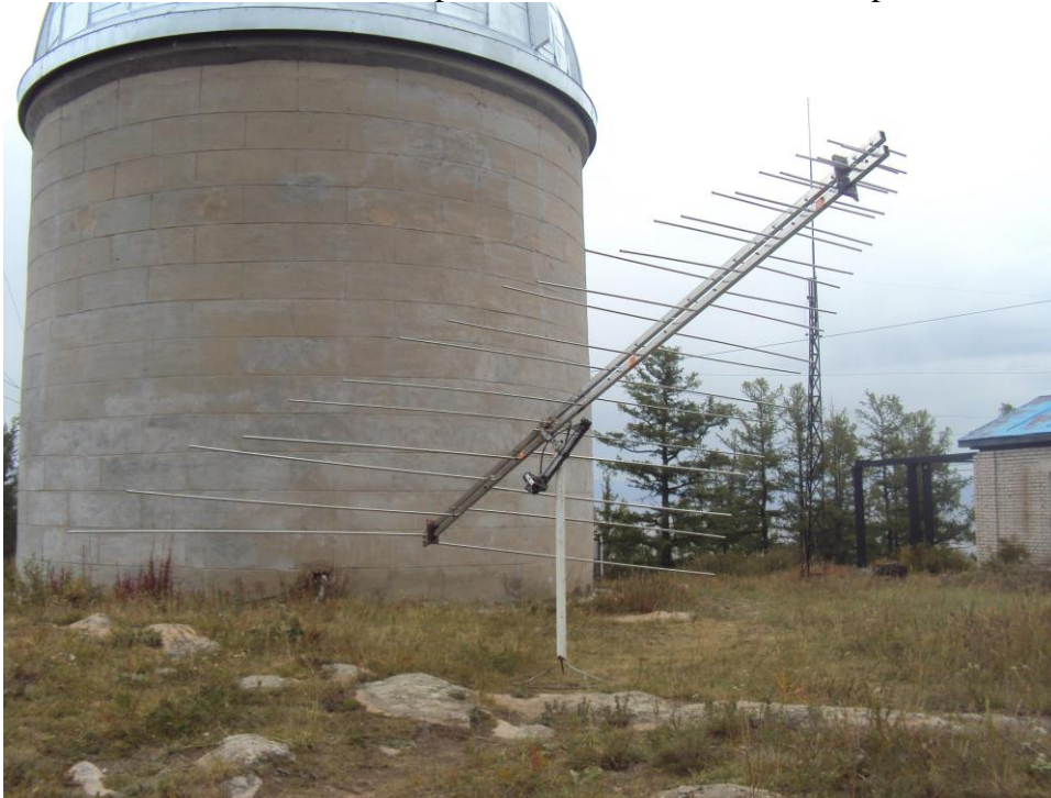
Fig. 5: Logarithmic periodic dipole array LPDA in front of an optical observatory in Mongolia.
