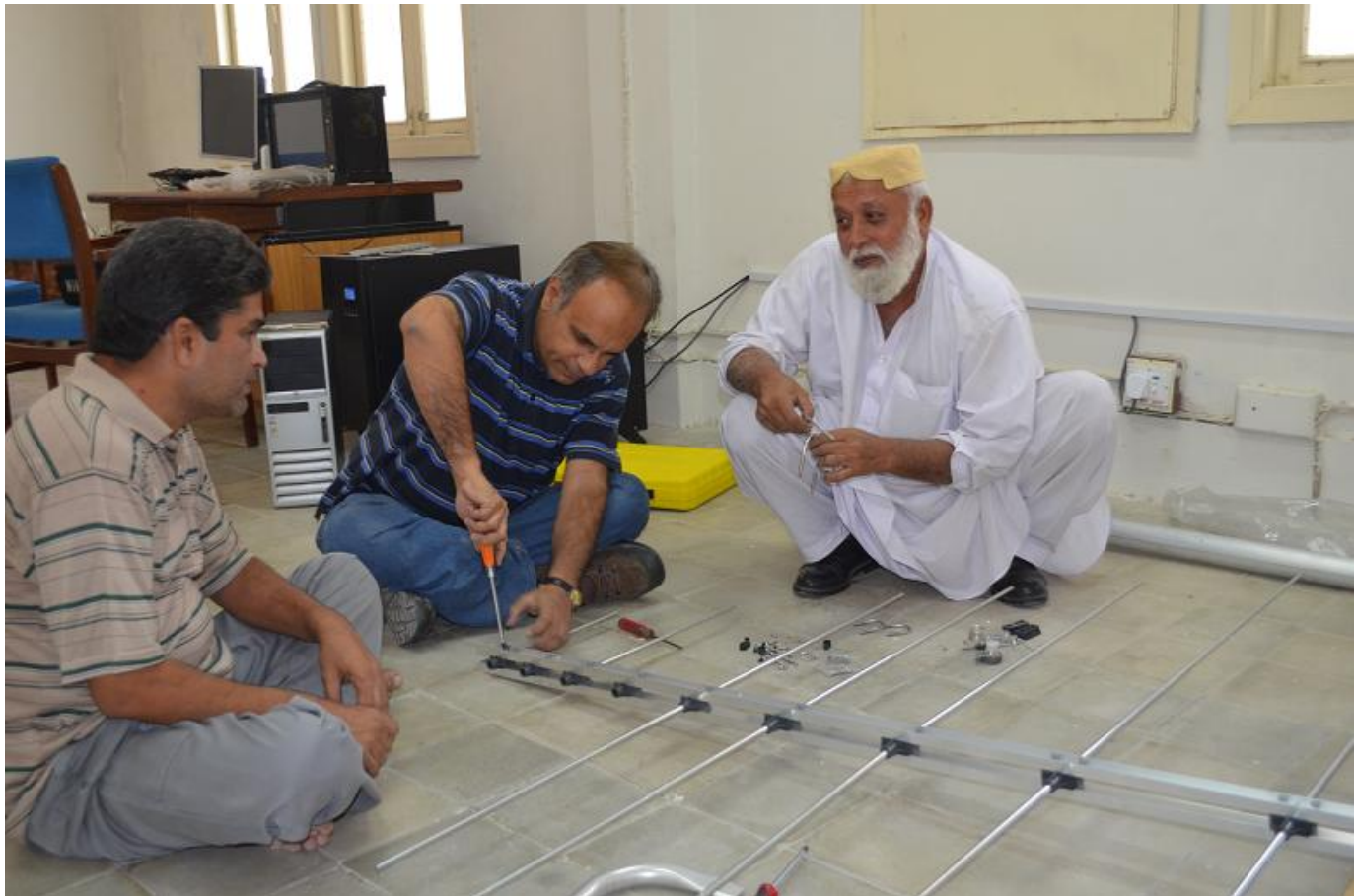
Fig. 3: Assembling of the logarithmic periodic dipole array LPDA at SUPARCO in Pakistan.
