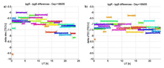
Fig. 2 Single differences of the levelled carrier-phase ionospheric observable (different *colours* correspond to different satellites). a Sites: lpgR and lpgB, day 188/05. b Sites: lpgR and lpgB, day 189/05
