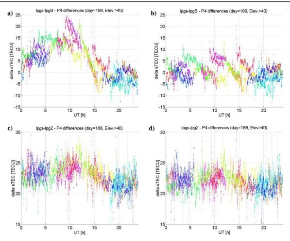
Fig. 3 Smoothed single differences of the code-delay ionospheric observable (different *colours* correspond to different satellites). a Sites: lpgs and lpgB, day 188/05. b Sites: lpgs and lpgB, day 189/05. c Sites: lpgs and lpg2, day 188/05. d Sites: lpgs and lpg2, day 189/05
