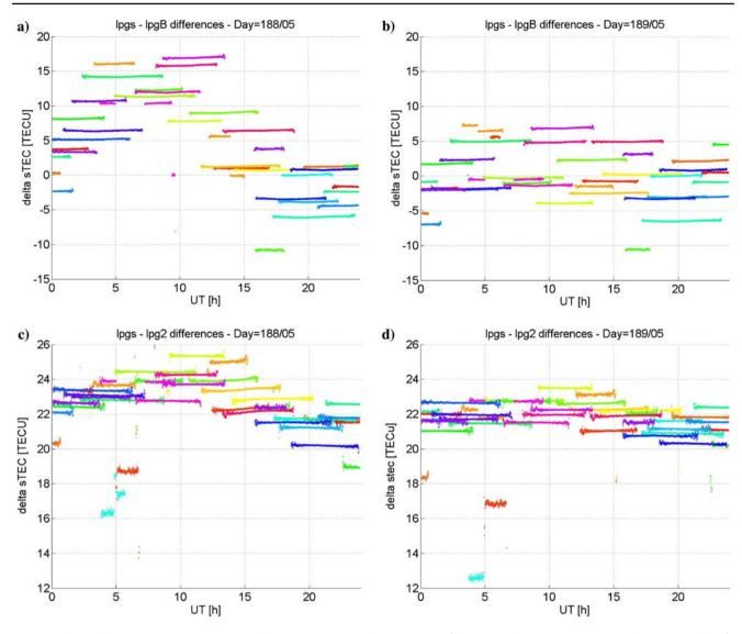
Fig. 1 Single differences of the levelled carrier-phase ionospheric observable (different *colours* correspond to different satellites). a Sites: lpgs and lpgB, day 188/05. b Sites: lpgs and lpgB, day 189/05. c Sites: lpgs and lpg2, day 188/05. d Sites: lpgs and lpg2, day 189/05
