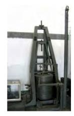
On 1 June 1937, the two horizontal seismographs (NS and EW) Mainka mass of 450 kg (Photo left) began recording, their period is about 12 s, and the records are on paper in black smoke. In the early sixties, a third vertical seismograph cal Grenet-Coulomb-type will be added to the other two. By the mid-seventies, the records will be in ink.
