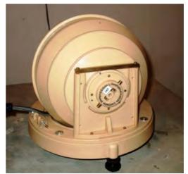
From April 2003, a new digital acquisition system geomagnetic data has been established. The control equipment of the geomagnetic field variations and the base lines consist of: 1) a magnetometer (fluxgate), mounted on theodolite (Type 010A Zeiss) and equipped with readout electronics,
