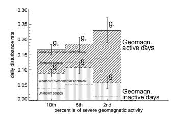
**Fig. 3.** Graphical rendition of the grid disturbance rates under different levels of geomagnetic activity, as listed in Table 1. The three columns show the results for geomagnetic activity in the 10th, 5th, and 2nd upper percentiles of geomagnetic activity as measured by |dB/dt(30m)|, respectively. The excess in event frequency on geomagnetically active days compared to nearby inactive days is shown by dark diagonal shading.
