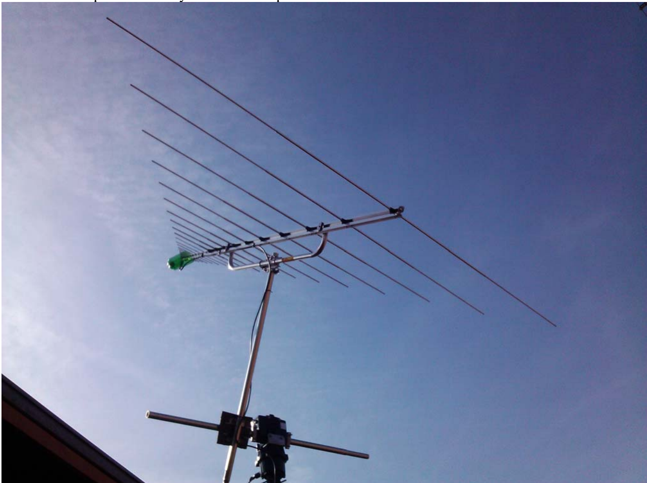
Fig. 1: The antenna is a commercial LPDA (Logarithmic Periodic Dipole Array) from CREATE CLP5130-1N connected to a low noise preamplifier Mini-Circuits ZX60-33LN with 20 dB of gain and 1.1 dB of noise figure. Data (EA4RKU*.fit) are already transferred in real time to the archive at FHNW in Switzerland. The antenna can track the sun with a radio-amateur positioning system.
