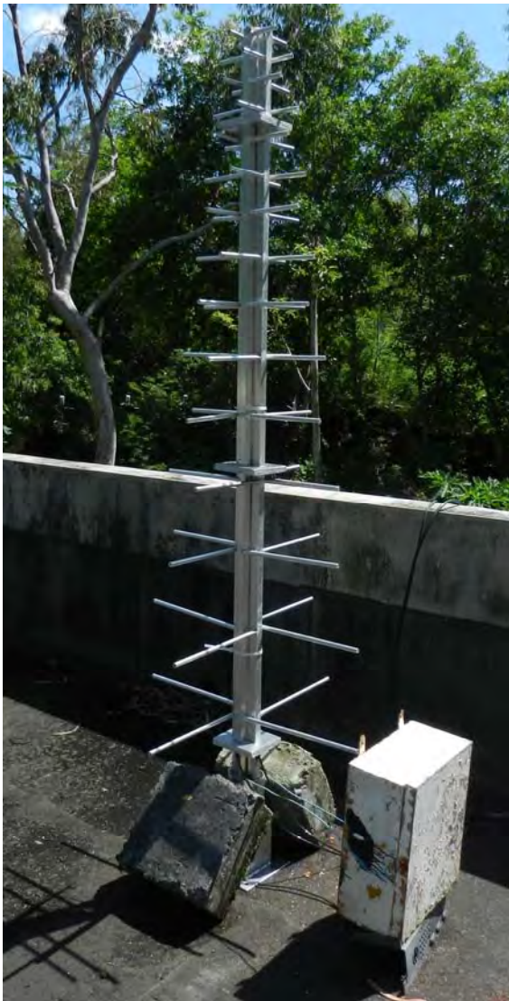
Fig. 3: log-per at MRT. In the background between the bushes some white helix antennas from the historic large interferometer at 150 MHz.
