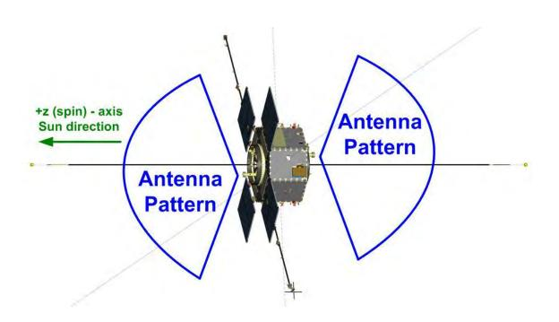
Figure 3: RBSP RF Antenna Covereage
