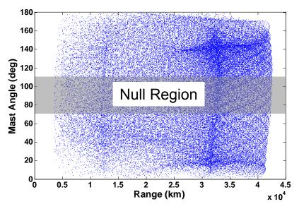
Figure 2: Required RBSP Antenna Angle Coverage
