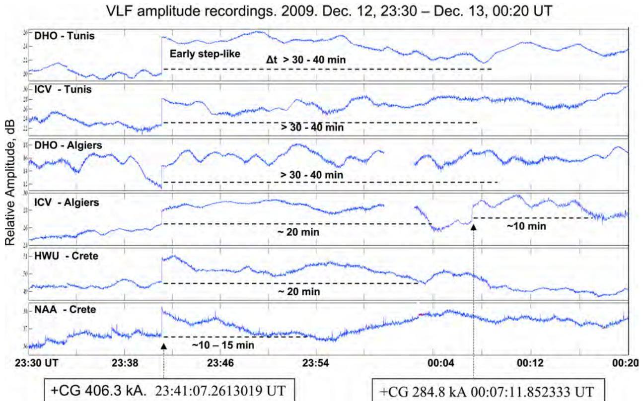
**Figure 3.** Step-like early VLF events corresponding to the elves shown in Figure 2, both triggered by very intense +CG lightning strokes. They are observed at by transmitter-receiver GCPs passing at relatively large distances from the causative lightning flashes. These type of early perturbations offset the transmission signal levels for long times. See text for more details.
