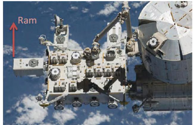
Fig. 5. The Japanese Experiment module has both ram and wake facing attachment points for exposed facilities (courtesy JAXA<sup>8)</sup>).
