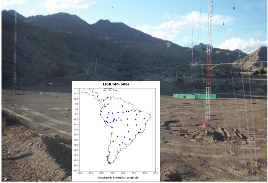
Figure 1. Antenna Field of the VIPIR ionosonde installed at Tupiza in Bolivia and a map of the Locations of the GPS deployed in South America (blue dots). contact: Cesar Valladeres – Boston College. cesar.valladares [at] bc.edu
