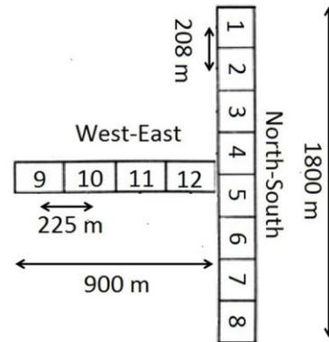
Figure 1. Scheme of the radio telescope UTR-2, which consists of 8 North-South sections and 4 West-East sections.
