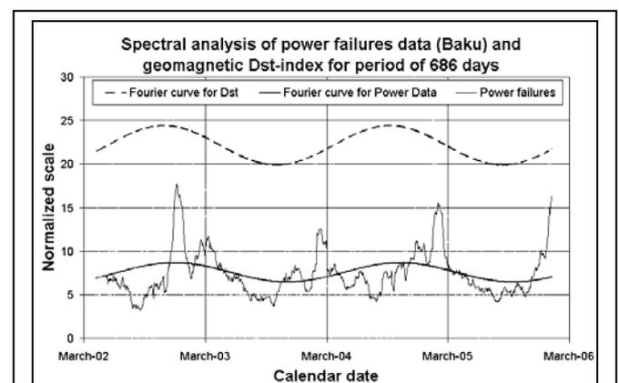
Fig.3. Spectral analyses of power supply system failures and Dst index for period of 686 days, Baku data.
