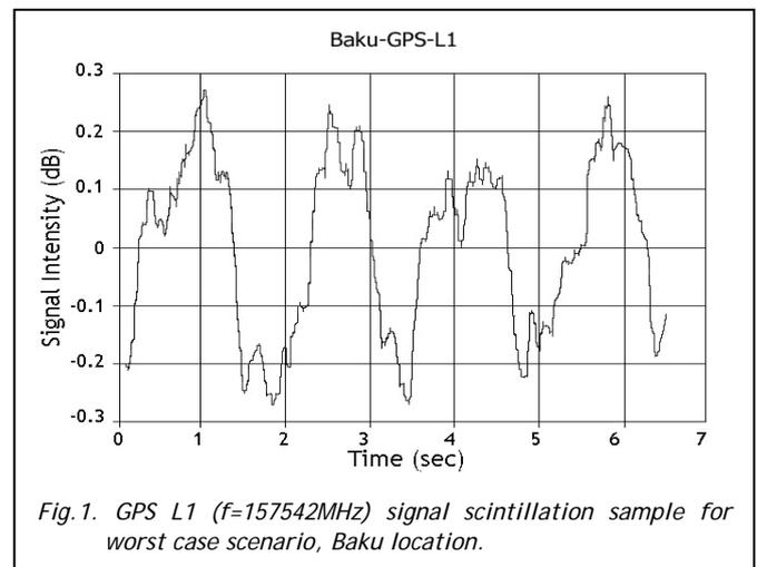
Fig.1. GPS L1 ( $f=157542$ MHz) signal scintillation sample for worst case scenario, Baku location.
