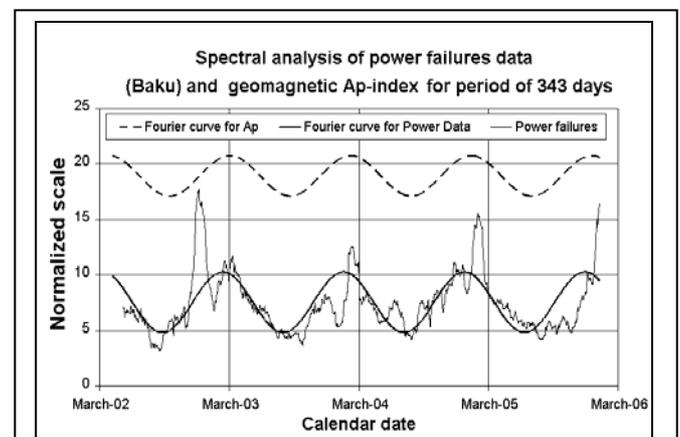
Fig.2. Spectral analyses of power supply system failures and Ap index for period of 343 days, Baku data.
