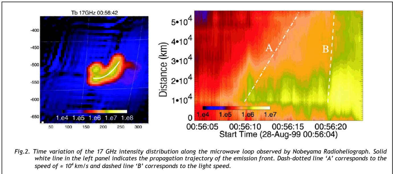
Fig.2. Time variation of the 17 GHz intensity distribution along the microwave loop observed by Nobeyama Radioheliograph. Solid white line in the left panel indicates the propagation trajectory of the emission front. Dash-dotted line 'A' corresponds to the speed of  $\approx 10^4$  km/s and dashed line 'B' corresponds to the light speed.
