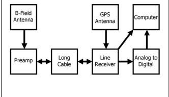
Fig.1. The block network of the system for monitoring, collecting and storing the data at the campus of the Sharjah University.
