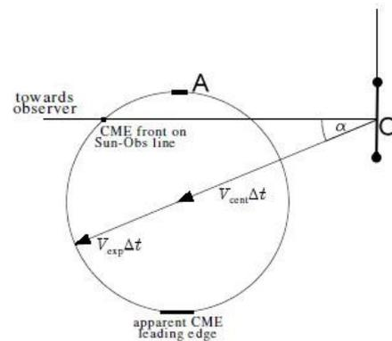
Fig. 2 A simple sketch of a spherical CME which expands self-similar. The center is assumed to propagate radially away from the Sun. The figure shows a meridional cut through the CME center.  $\alpha$  is the propagation latitudinal angle. Adapted from Srivastava et al. (2009).
