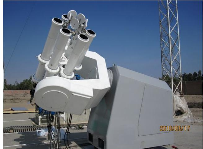
Figure 2 Flare Monitoring Telescope (FMT) at National Ica University, Peru
